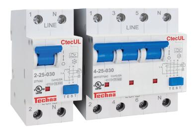
The CtecUL series of Equipment Ground Fault Protection Relays (Earth Leakage Protection) is the latest addition to Techna's UL Listed product range, providing ground fault (residual current) protection for circuits with loads up to 63A with a short circuit interrupting capacity of 10kA.
